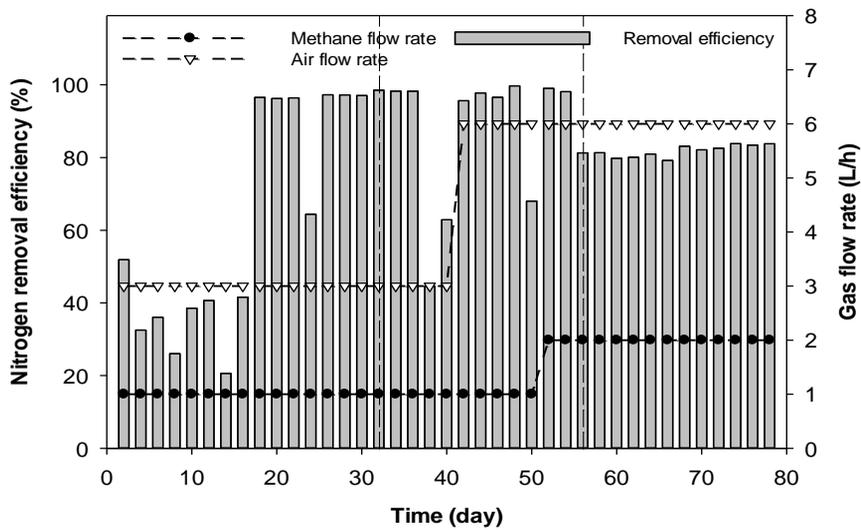
Figure 4. Removal efficiency with different gas flow rate.
