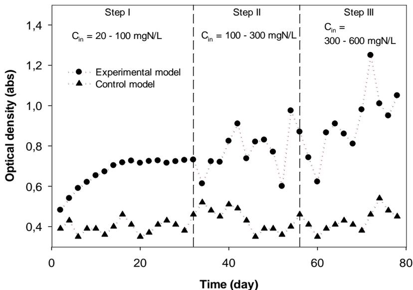
Figure 2. Microbial density in AMO-D bioreactor.
