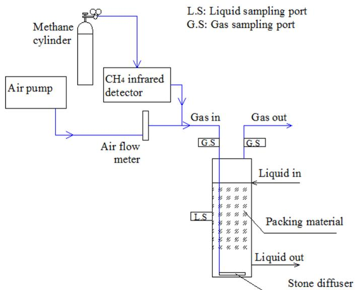
Figure 1. AMO-D bioreactor with methane and air supplied together.
