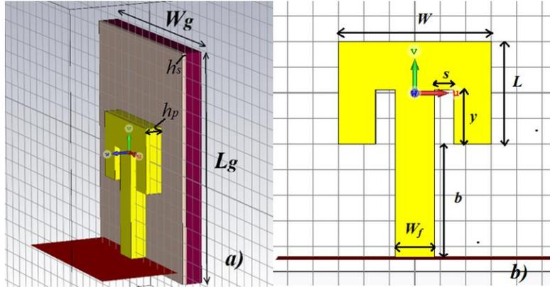
Figure 1. The geometrical structure of the proposed antenna: side view (a) and top view (b).
