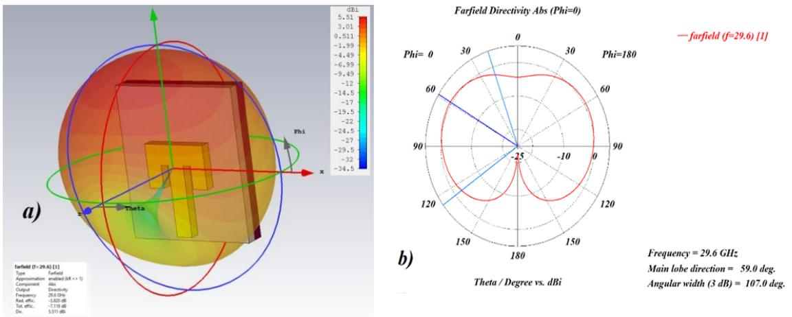
Figure 3. 3D directivity patterns (a) and 2D directivity patterns (b) of the proposed antenna at 29.6GHz.
