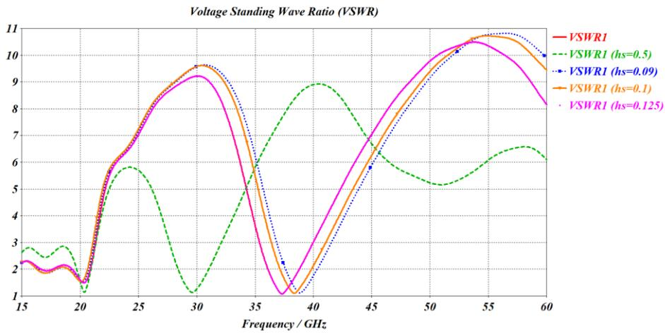
Figure 5. Simulated VSWR-parameters of different substrate's thickness  $h_s$ .
