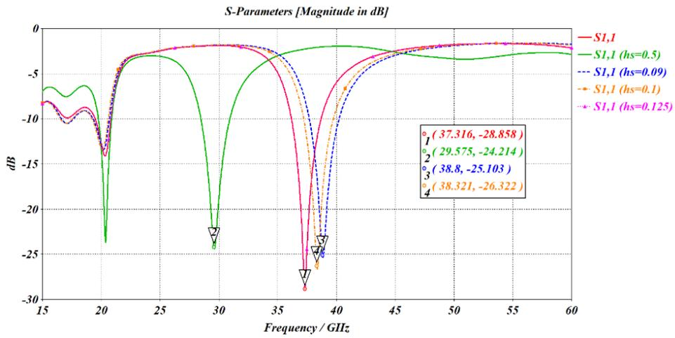
Figure 4. Simulated S-parameters of different substrate's thickness  $h_s$ .
