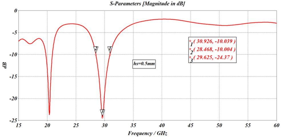
Figure 2. The plot of  $S_{11}$  parameters for the proposed antenna at 28 GHz bands.
