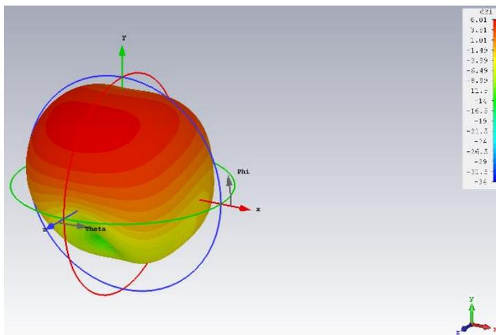
Figure 6. Simulated directivity patterns of proposed 5G antenna at frequency 38 GHz.
