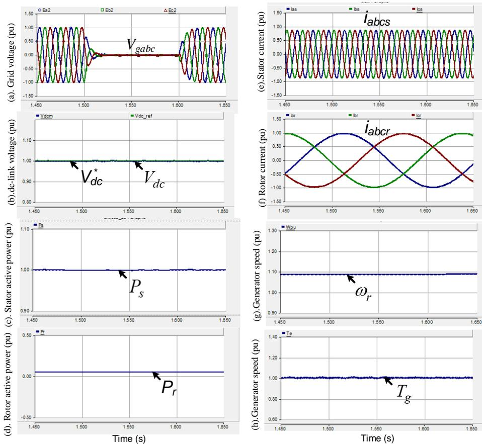
Figure 7. Performance of DFIG wind turbine system for three-phase voltage interruption (in pu).
