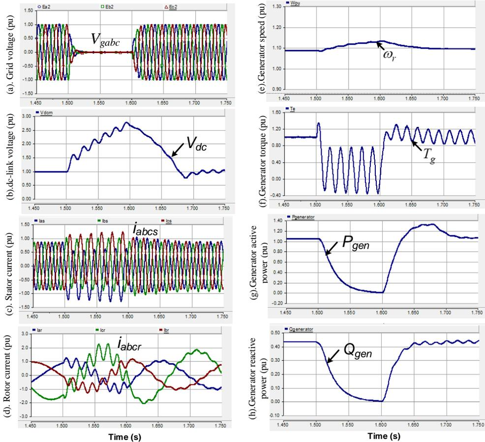
Figure 4. Performance of DFIG wind turbine system for the three-phase voltage interruption (in pu).
