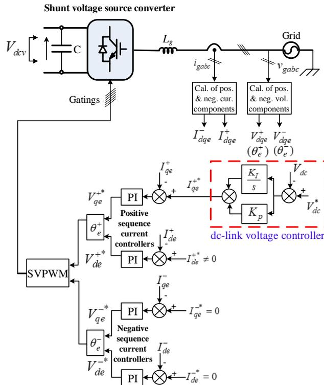
Figure 3. Control block diagram of a shunt VSC.
