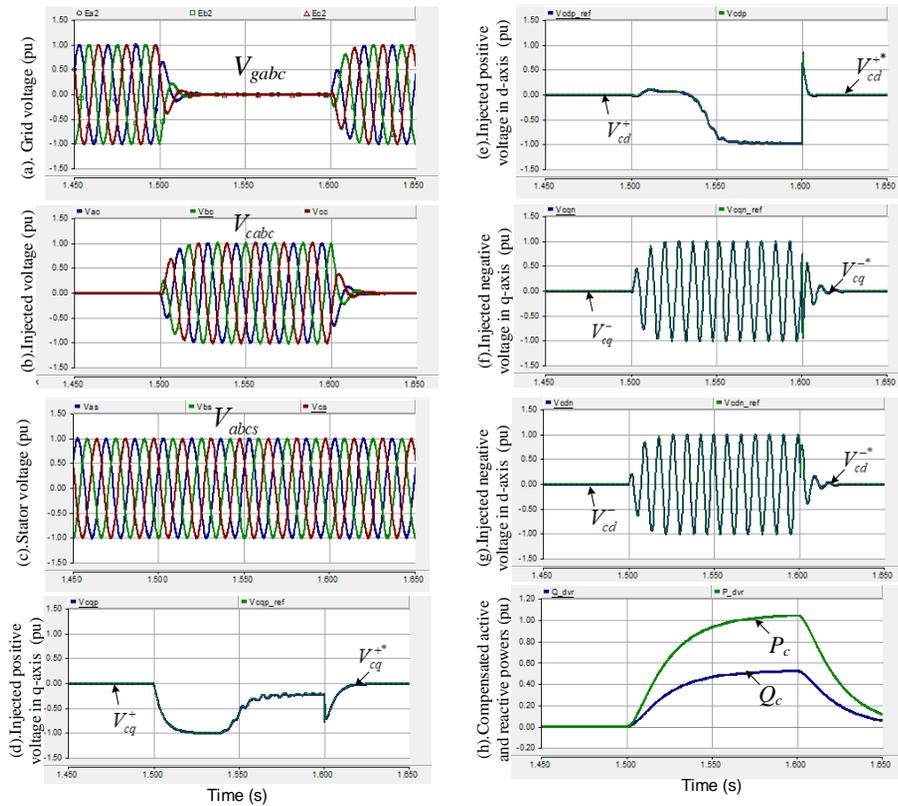
Figure 5. Performance of series VSC for the three-phase voltage interruption (in pu).
