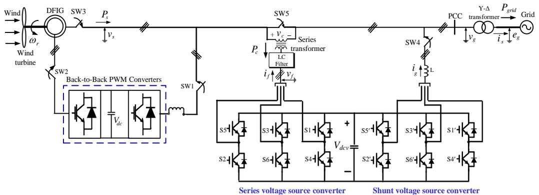
Figure 1. Circuit configuration of DFIG wind turbine systems with two VSCs.
