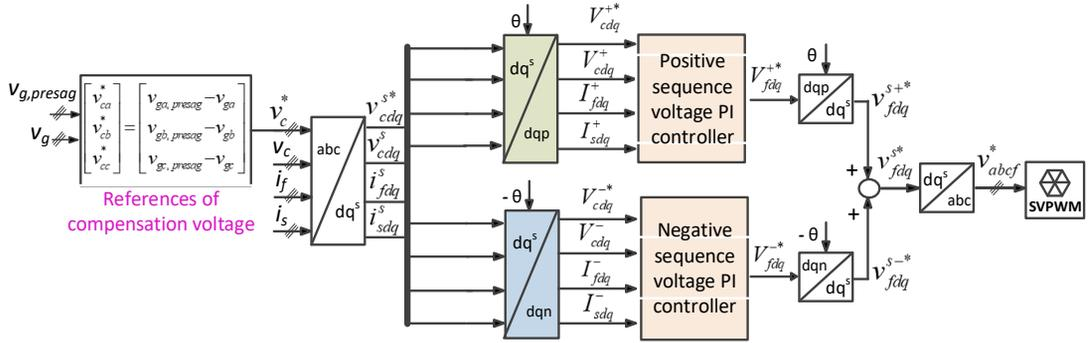
Figure 2. Control block diagram of a series VSC.
