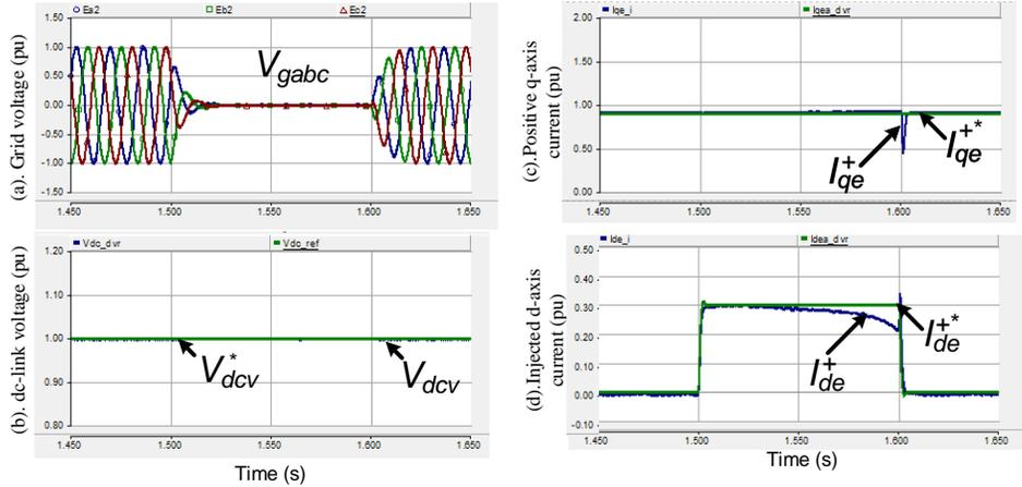
Figure 6. Performance of shunt VSC for the three-phase voltage interruption (in pu).
