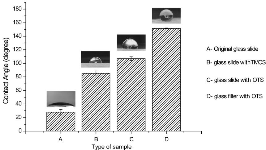
Figure 5. Change of contact angle values by chemical treatment.
