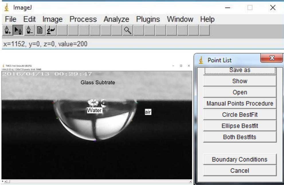
Figure 3. Points picking on water droplet
