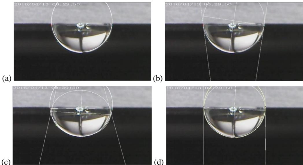
Figure 4. Fitting droplet curve using ImageJ with (a) circle best-fit; (b) ellipse best-fit; (c) both best-fit; (d) manual point procedure.
