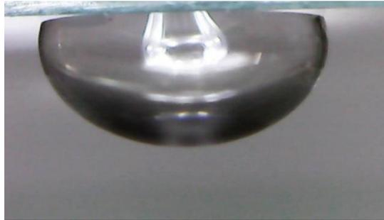
Figure 1. Water droplet image on OTS-treated glass slide captured using picture function of Koolertron microscope.
