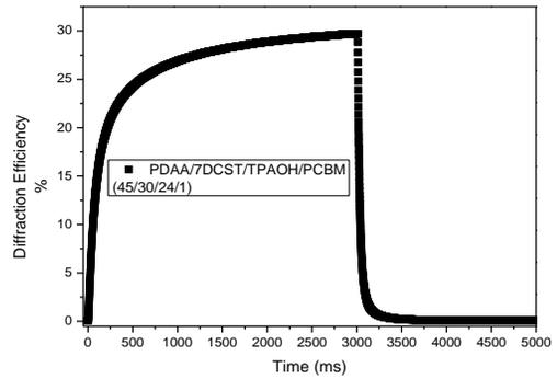
Figure 6. Diffraction efficiency as the function of time of the composite PDAS/7DCST/TPAOH/PCBM (45/30/24/1)
