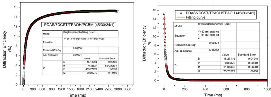
Figure 5. Rising and decaying of diffraction efficiency signal for PDAS based PR composite
