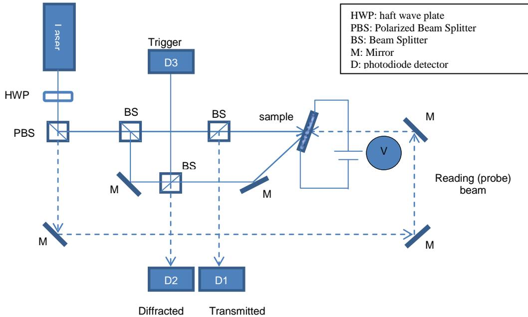
Figure 3. Optical geometry for DFWM
