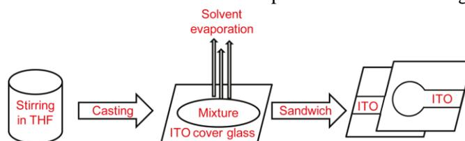
*Figure 2.* PR cells fabrication
