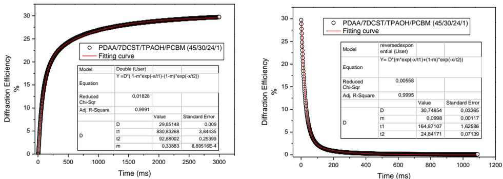
Figure 7. Rising and decaying of diffraction efficiency signal for PDAA-based PR composite
