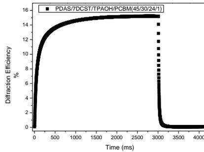
Figure 4. Diffraction efficiency as the function of time of the composite PDAA/7DCST/TPAOH/PCBM (45/30/24/1)
